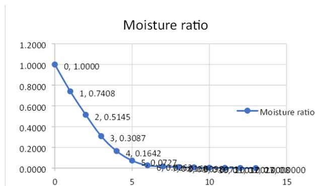
**Fig. 3.** Drying characteristics of jaggery treated banana at 50°C
