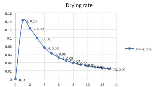
**Fig. 4.** Drying rate characteristics of sugar treated banana at 60°C.
