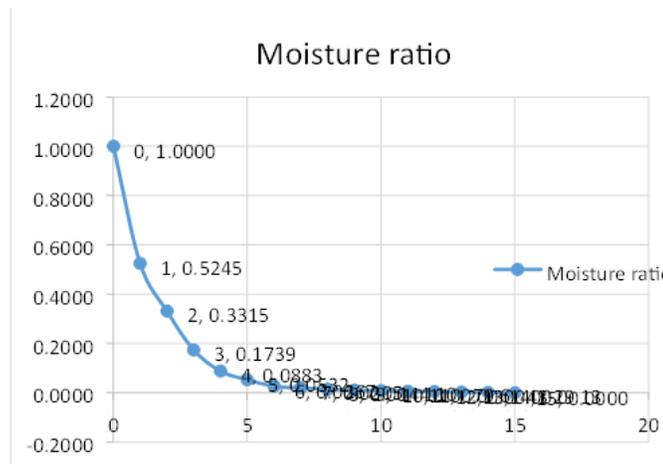
Fig. 1. Drying characteristics of control banana at 50°C
