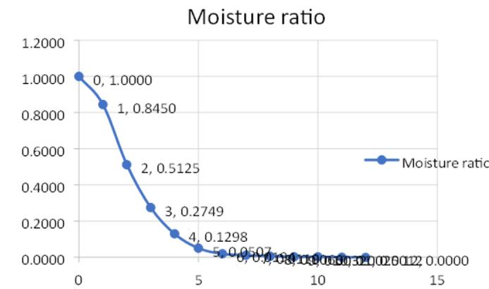
Fig. 2. Drying characteristics of sugar treated banana at 50°C
